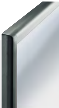
20650 ROVAL™ STAINLESS STEEL MIRROR 20655 ROVAL™ STAINLESS STEEL MIRROR WITH INTEGRAL SHELF Gently radiused edges match the ASI Roval™ design. Frame fabricated of 18 gauge type 304 stainless steel with satin finish and polished seamless mitered corners. 0.25" (6.4 mm) thick plate glass mirror.
