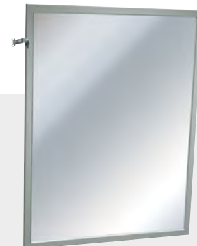
0600-T ADJUSTABLE TILT MIRROR Designed to provide easy visibility for wheelchair patients or return to upright position. Angle frame fabricated of 18 gauge stainless steel with corners welded and ground smooth. Tilts a full 6" (152 mm) with bottom mounted on full width stainless steel piano hinge.
