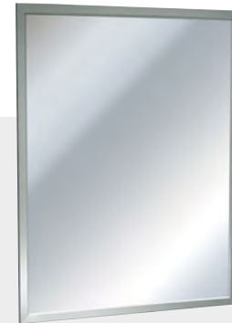
0600 ANGLE FRAME MIRROR 3/4" x 5/8" (19 x 16 mm) roll formed 18 gauge type 304 stainless steel angle has corners heliarc welded, ground and polished smooth to a uniform satin finish. Mirror is installed on a concealed hanging bracket that locks onto top and bottom of frame by tamper-proof set screws. Back plate is one-piece, attached to frame with theft-resistant locking device.
