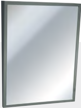
0535 FIXED TILT MIRROR Offers visibility for wheelchair patients. Frame fabricated of 20 gauge stainless steel with a satin finish. Mirror is tapered from 4" (102 mm) at top to 1" (25 mm) at bottom.
